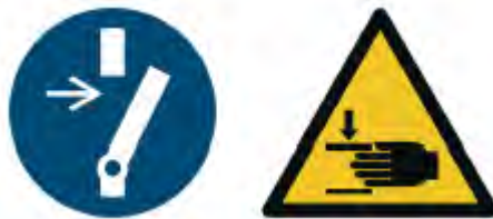
66947 – Mandatory sign/warning sign: Completely disconnect/warning of hand injury
