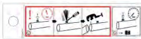
940 – Warning “Transport filling” on the Schrader valve
